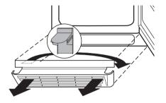
With the freezer compartment door closed, remove the crosshead screws from the lower door bearing and remove the door bearing downwards.
